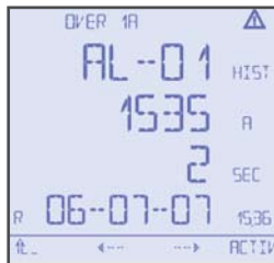
Alarm display showing active alarm
