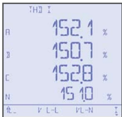
Current total harmonic distortion display
